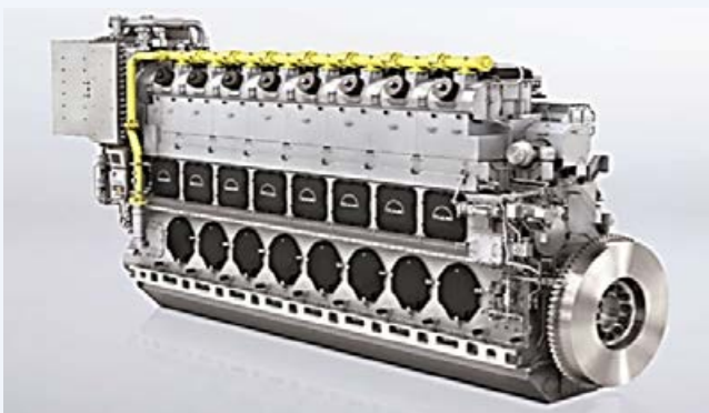
Slika 13: Pogled na MAN 8L51/60DF Picture Credits: marine.mandieselturbo.com
